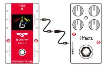
Attention: Incorrect polarity would damage this unit, please make sure correct positive and negative polar before wiring.
